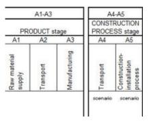
The value stated in the EPD for 1 Cody chair is calculated for A1-A4, which stands for raw materials (A1 which applies to everything from resource extraction to products to be used in the chair Cody), transport to Sykkylven (A2), manufacturing at Sykkylven Stål (A3), and transport to the customer/or inventory (A4).
